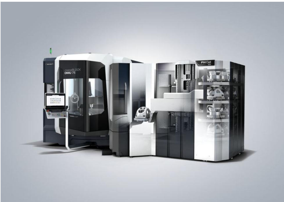
The modular PH Cell 500 offers space for up to 32 pallets, each measuring 400 x 400 mm. The rotating set-up station and touchscreen control ensure a high level of ergonomics and simple operation.
