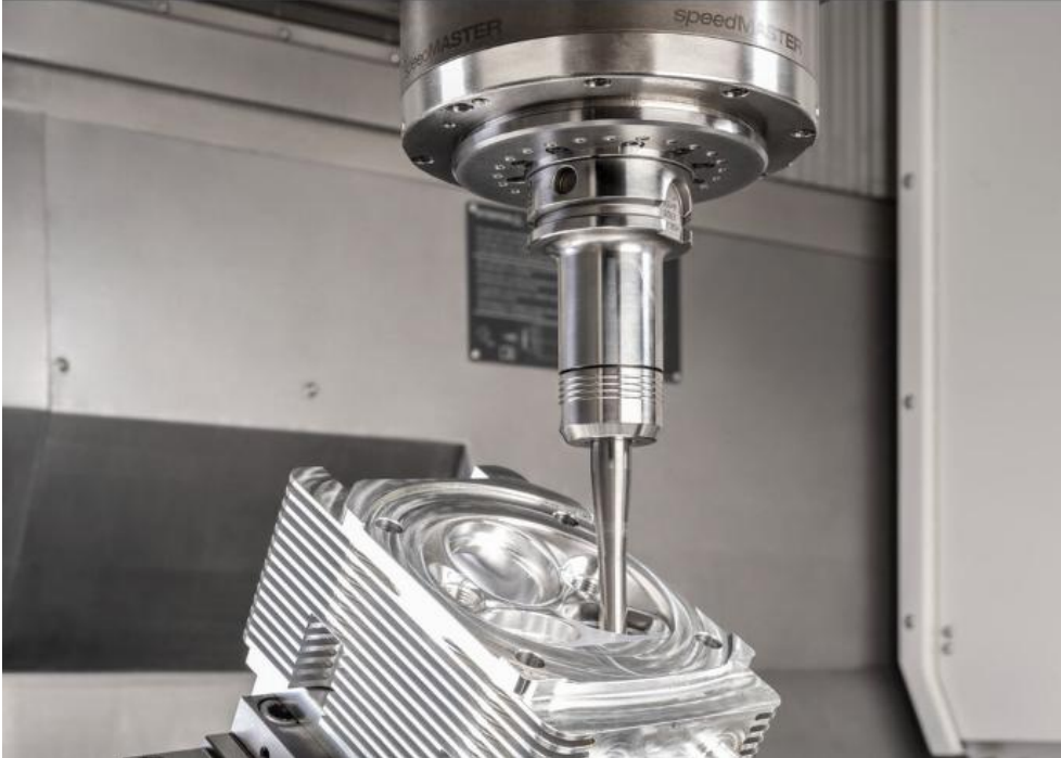
Machining of an engine block on the DMU 75 monoBLOCK with PH Cell 300.
